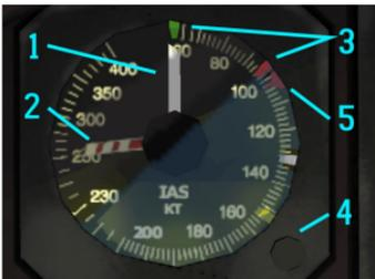
Figure 38: Airspeed indicator
