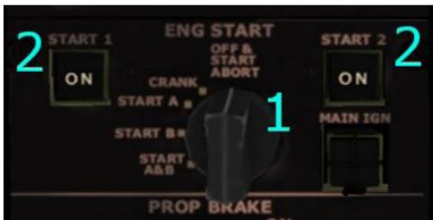
Figure 72: Engine start panel
