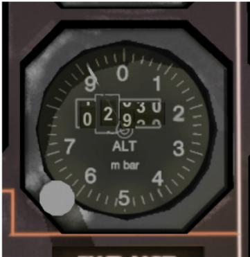
Figure 41: Standby altimeter
