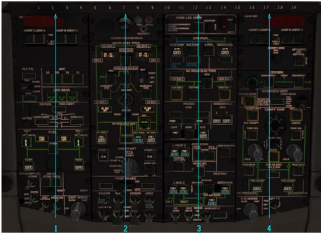
Figure 6: Overhead panel scan sequence
