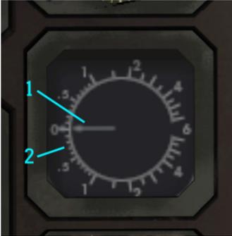
Figure 42: Vertical speed indicator
