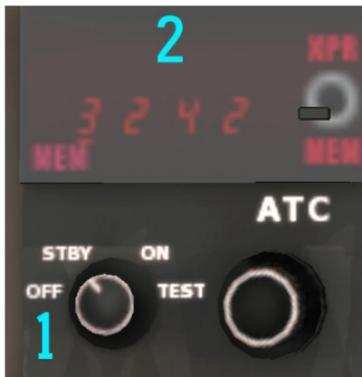
Figure 24: ATC control box
