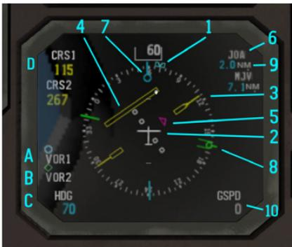
Figure 47: Electronic Horizontal situation indicator
