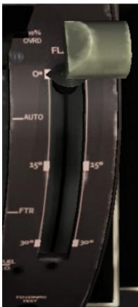
Figure 37: Flaps control lever
