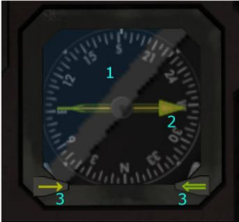
Figure 44: Radio magnetic indicator
