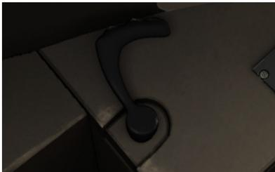
Figure 61: Nose Wheel steering
