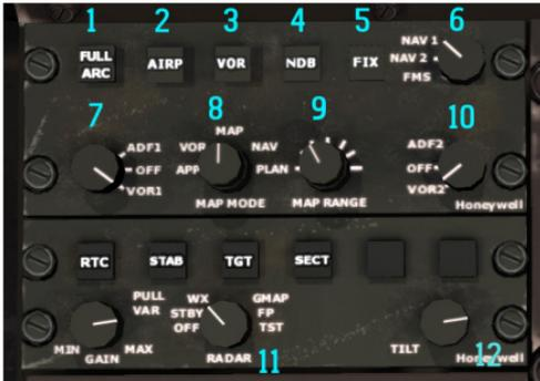
Figure 49: EFIS control panel
